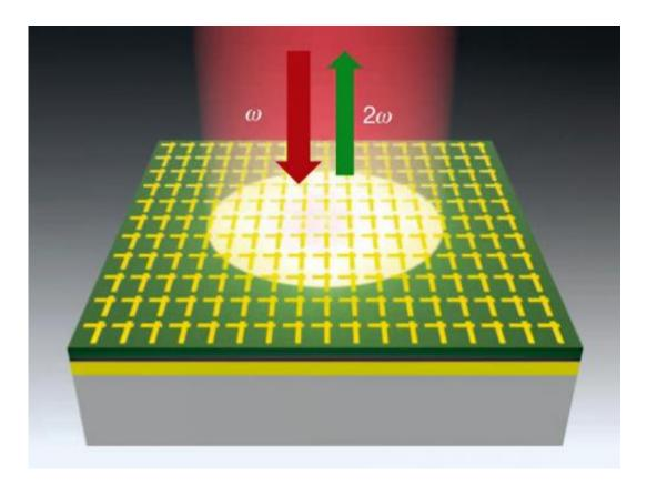
This is the 400-nanometer-thick nonlinear mirror that reflects frequencydoubled output using input light intensity as small as that of a laser pointer. Credit: University of Texas, Austin
