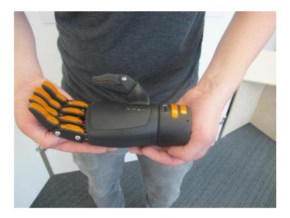
The arm would be controlled through the use of electromyography, a system used for many <u>artificial limbs</u>. Three electrodes will run from the Myo hand to the real upper arm of the amputee, who would be taught to control the prosthetic hand using the upper arm's individual muscle movements.
