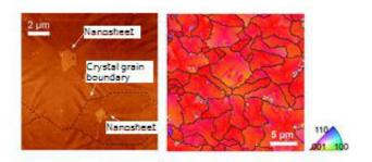
Figure 1 (left) An atomic force microscope image of the titanium oxide thin film fabricated by the new method, showing that nanosheets, which provided seed crystals, exist at the center of crystal grains. (right) A map of crystal grain orientation determined by electron backscattering diffraction. The black lines correspond to the boundaries of individual crystal grains and the color represents their orientation. All crystal grains are highly (001) oriented.
