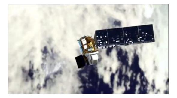
Every full moon, Landsat 8 turns its back on Earth. As the satellite's orbit takes it to the nighttime side of the planet, Landsat 8 pivots to point at the moon. It scans the distant lunar surface multiple times, then flips back around to continue its task of collecting land-cover information of the sunny side of Earth below.
