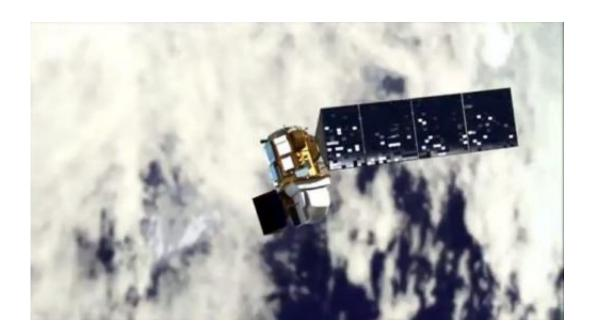
Every full moon, Landsat 8 turns its back on Earth. As the satellite's orbit takes it to the nighttime side of the planet, Landsat 8 pivots to point at the moon. It scans the distant lunar surface multiple times, then flips back around to continue its task of collecting land-cover information of the sunny side of Earth below.
