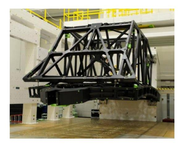
The backplane of NASA's James Webb Space Telescope was mounted to a structure for static load testing to verify it can withstand the rigors of launch and hold the weight needed to support the telescope in space. Credit: Northrop Grumman
