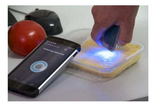
In this Wednesday, May 28, 2014 photo, a man works with a pocket-sized scanner called SCiO at the Consumer Physics laboratory near Tel Aviv, Israel. The scanner can identify the molecular structure of a substance by shining an infrared light on an object and reading its chemical makeup. It can then send additional information to a smartphone. (AP Photo/Jon Gerberg)
