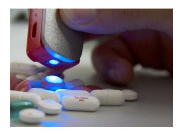
In this Wednesday, May 28, 2014 photo, a man works with a pocket-sized scanner called SCiO at the Consumer Physics laboratory near Tel Aviv, Israel. The scanner can identify the molecular structure of a substance by shining an infrared light on an object and reading its chemical makeup. It can then send additional information to a smartphone. (AP Photo/Jon Gerberg)
