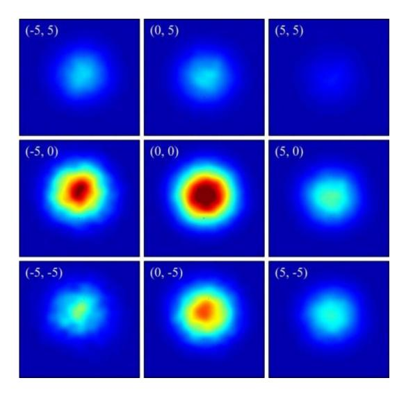
These are nearfield intensity profiles of a fibre measured with the UV beam coming from different directions. These profiles show that the light is single-mode. Credit: PTB
