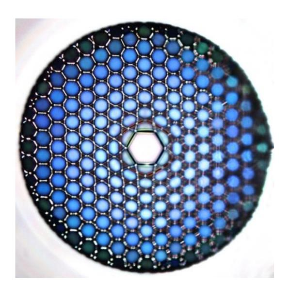
A microscopic image of a hollow-core optical fiber. Credit: : MPL
