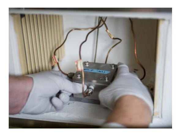
This close-up photograph shows the prototype reactor module used to fabricate hollow-fiber metal-organic framework membranes at Georgia Tech using the interfacial microfluidic technique. Credit: Rob Felt
