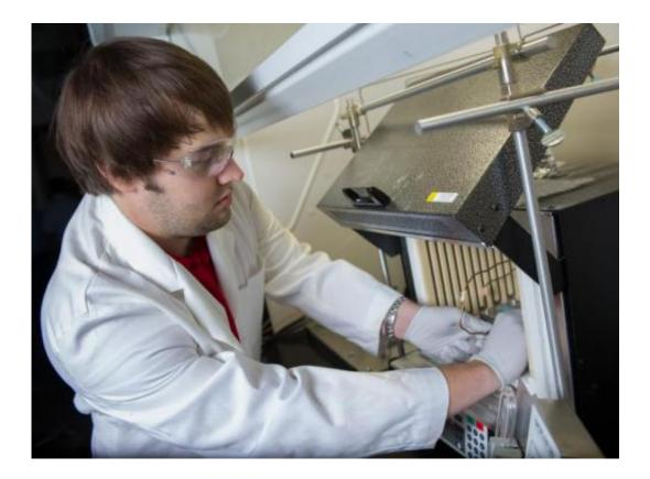
Georgia Tech researcher Andrew Brown places a finished hollow fiber metalorganic framework membrane module into a membrane testing apparatus to measure its gas separation properties. Credit: Rob Felt
