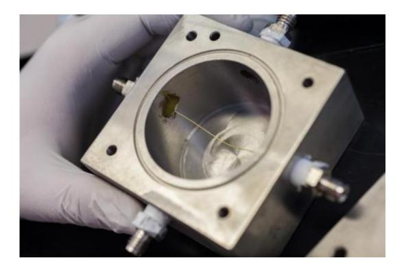
This photograph shows the inside of the prototype hollow-fiber metal-organic framework membrane module, revealing a hollow fiber MOF membrane mounted in it. Credit: Rob Felt
