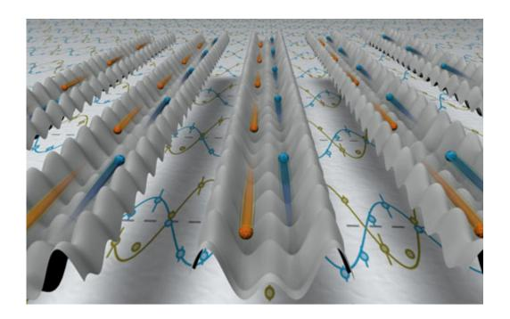
Schematic representation of the light crystal with ladder-like shape. The blue and yellow spheres represent the atoms traveling in opposite directions, as in the Meissner phase. In the experiment the strength of the current was measured, which indicated a transition from the vortex to the Meissner phase. Credit: MPQ, Quantum Many Body Systems Division
