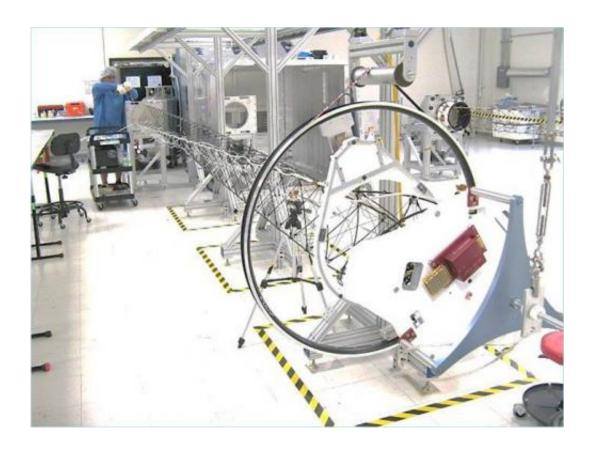
This image captures the first functional deployment of the Magnetometer boom. Credit: ATK/Goleta
