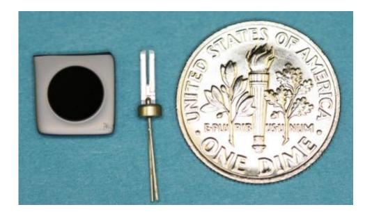
Vahala's new laser frequency reference (left) is a small 6 mm disk; the quartz "tuning fork" (middle) is the frequency reference commonly used today in wristwatches to set the second. The dime (right) is for scale. Credit: Jiang Li/Caltech
