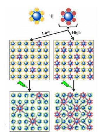
When low concentrations of crosslinker are added to the resist (left), it is able to pattern smaller features and doesn't require longer, expensive exposures as with a high concentrations of crosslinker (right). Credit: Prashant Kulshreshtha, Berkeley Lab
