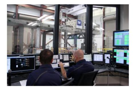
The state-of-the-art control room in the University of Nevada, Reno's new expanded Earthquake Engineering Laboratory operates all the systems in the world-renowned facility, from the massive hydraulics that power the four 14- by 14-foot 50-ton capacity shake tables to the 400 sensors that gather data on the experiments that sit atop the tables. the first multi-shake-table experiment in the lab can be see in the background. Credit: Mike Wolterbeek, University of Nevada, Reno.
