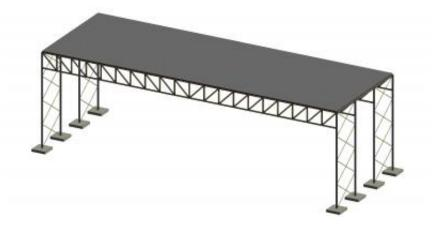
This is a pratt truss structural system for Functional Unit 2 (3 bays or units). Credit: ASCE
