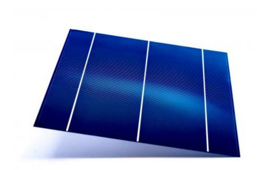
Nano-electronics research center imec, reported today an n-type PERT crystalline silicon (Si) solar cell fabricated on a large area wafer (15.6cm x 15.6 cm) reaching a top conversion efficiency of 21.5 percent (calibrated at ISE Callab). This is the highest efficiency achieved for this type of solar cell on an industrial large area wafer size. This result will
