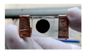
Zinc porphyrin dyes were used to create solar cells that can absorb both visible and near-infrared light. Credit: A\*STAR Institute of Materials Research and Engineering
