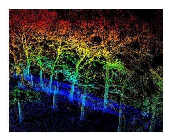
Digital three-dimensional model of forest trees generated by Dr. Sorin Popescu with the terrestrial lidar scanner. The color is associated with elevation above ground. Credit: Dr. Sorin Popescu
