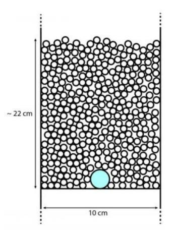
Schematic diagram of a cross-section of the experiment after an infinitely long cylindrical container (with a diameter of 10 cm) is filled up with small particles (up to  $\sim 22$  cm from the origin), but before shaking begins. The large cyan particle (the intruder) is initially located at the floor. Credit: arXiv:1407.2748 [astro-ph.EP]
