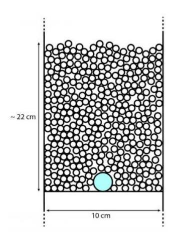
Schematic diagram of a cross-section of the experiment after an infinitely long cylindrical container (with a diameter of 10~cm) is filled up with small particles (up to  $\sim 22~\text{cm}$  from the origin), but before shaking begins. The large cyan particle (the intruder) is initially located at the floor. Credit: arXiv:1407.2748 [astro-ph.EP]
