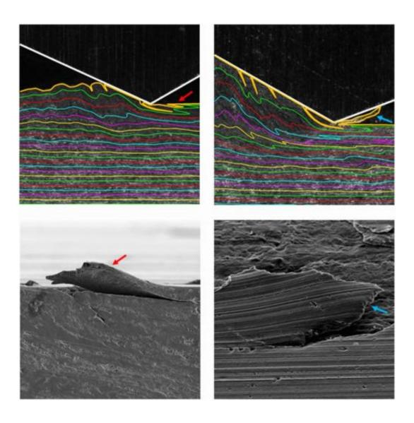
This sequence of images reveals surprising fluid-like behavior in a solid piece of metal sliding over another, forming defects leading to wear in metal parts. (Top) Two image frames of the material flow showing how these defects are spawned in the wake of the contact. (Bottom) Scanning electron microscope pictures of
