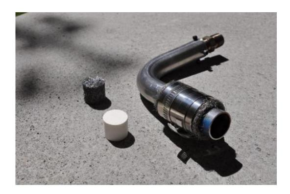
This is the device, with the stainless steel mesh filter and catalyst support structure detached. Credit: UC Riverside
