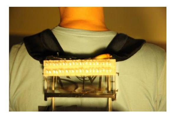
A new device harnesses the energy created by natural human walking to simultaneously light more than 40 commercial LEDs. The technology could revolutionize the way we charge small electronic devices, reducing dependence on non-renewable power sources and untethering users from fixed charging stations. Credit: Zhong Lin Wang, Georgia Tech.
