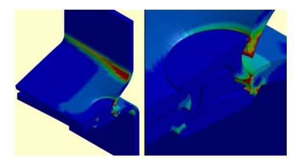
A punch-riveted joint fails under bending load: the red areas were particularly seriously deformed. Credit: Fraunhofer IWM
