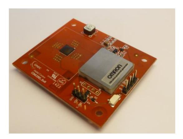
OMRON and Holst Centre/imec have unveiled a prototype of an extremely compact vibrational energy harvesting DC power supply with worlds' highest efficiency. The prototype will be demonstrated at the
