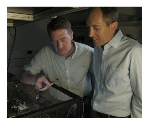
This image depicts NIST physicists Scott Diddams (left) and Scott Papp with a prototype atomic clock based on a chip-scale frequency comb. Diddams is holding the silicon chip, which fits into the clock apparatus on the table. With performance improvements and further reductions in size, the technology might eventually be used to make portable tools for measuring time and frequency. Credit: Burrus/NIST
