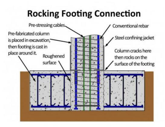
This graphic illustrates a new design for the framework of columns and beams that support bridges, called "bents," to improve performance for better resistance to earthquakes, less damage and faster on-site construction. The faster construction is achieved by prefabricating the columns and beams off site and later erecting and connecting them quickly at the construction site. Credit: University of Washington, Seattle/NEES photo
