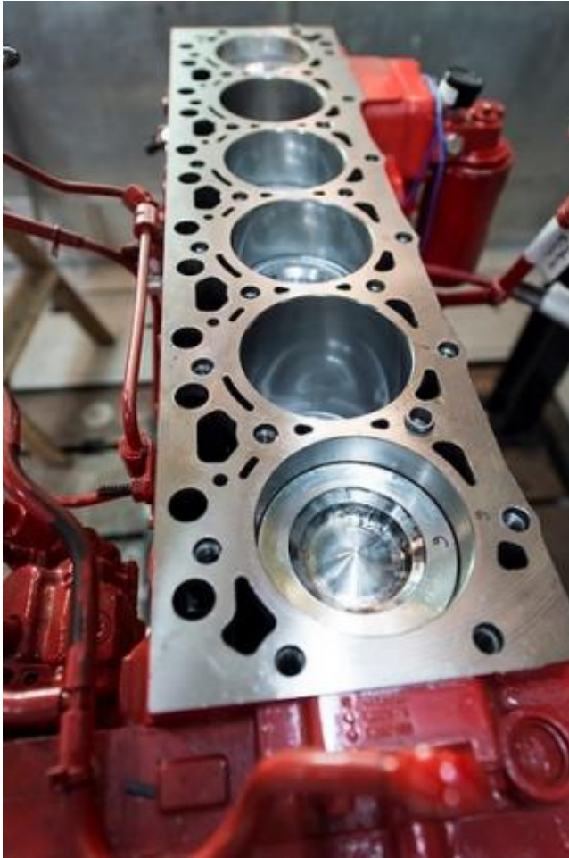
Bored cylinders in an open engine block are pictured at the Caterpillar Engine Lab. Credit: Jeff Miller
