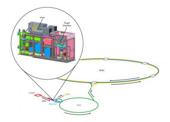
The Laser Ion Source feeds beams into RHIC and NSRL.
