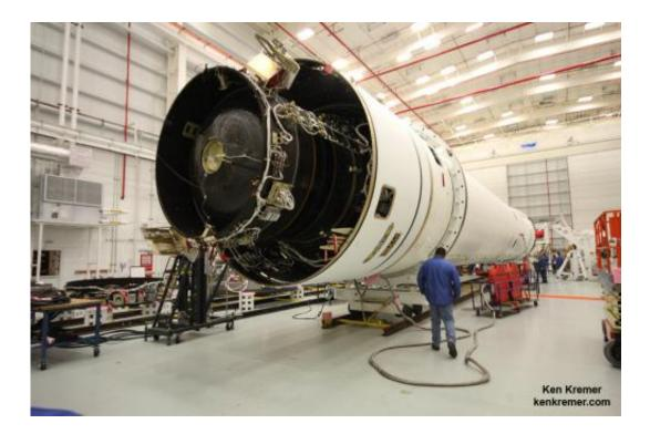
1st and 2nd stage of Orbital Sciences Antares rocket set for blast off on July 11, 2014 on the Orb-2 mission from NASA's Wallops Flight Facility in Virginia, bound for the ISS. The rocket undergoes processing at the Horizontal Integration Facility at NASA Wallops during visit by Universe Today/Ken Kremer. Credit: Ken Kremer
