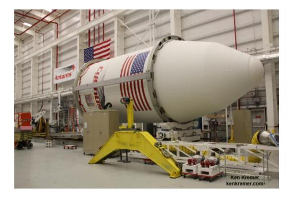
Up-close side view of payload fairing protecting Cygnus cargo module during launch for Orb-2 mission to ISS. Vehicle undergoes prelaunch processing at NASA Wallops during visit by Universe Today/Ken Kremer. Credit: Ken Kremer
