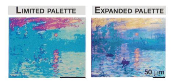
(Phys.org) —A team of researchers in Singapore has used plasmonic properties to create a photorealistic printing technique. In their paper published in *Nano Letters*, the researchers describe how they created pillars of hydrogen silsequioxane 95nm tall on a silicon substrate, each topped with an aluminum cap to take advantage of plasmon resonance, resulting in a printing palette of over 300 colors.
