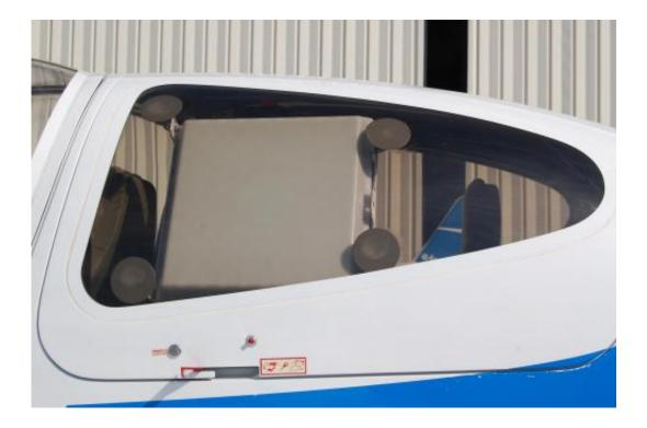
An Agile Aperture Antenna is shown in the window of an aircraft for a recent test flight. The software-defined, electronically-reconfigurable antenna can change beam directions in a thousandth of a second. Its light weight and low power requirements make it ideal for use in UAVs. Credit: GTRI photo
