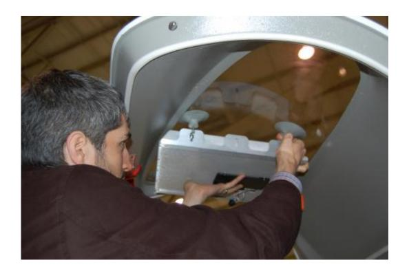
An Agile Aperture Antenna is placed in a window of an aircraft for a recent test flight. The software-defined, electronically-reconfigurable antenna can change beam directions in a thousandth of a second. Its light weight and low power requirements make it ideal for use in UAVs. Credit: GTRI photo
