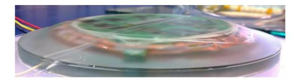
Interrogator (diameter 10cm) after embedding in protective epoxy shell with shape optimized for minimal impact on composite structural strength.
