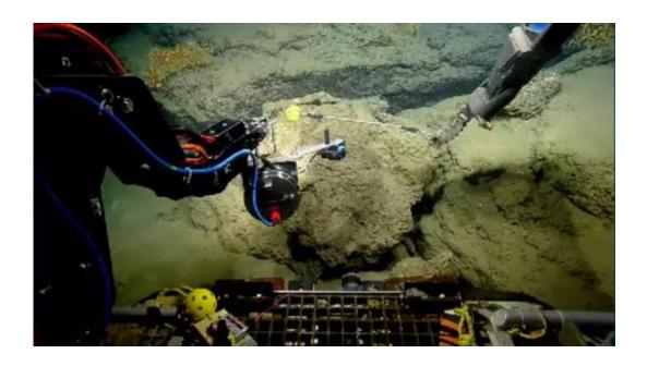
The remotely operated vehicle (ROV) Hercules working on the ocean floor. Credit: Sea Research Foundation, Inc.
