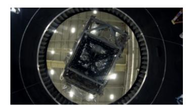
(Phys.org) —Engineer Jack Marshall held his breath. The "heart" of the James Webb Space Telescope hung from a cable 30 feet in the air as it was lowered slowly into the massive thermal vacuum chamber at NASA's Goddard Space Flight Center in Greenbelt, Maryland.
