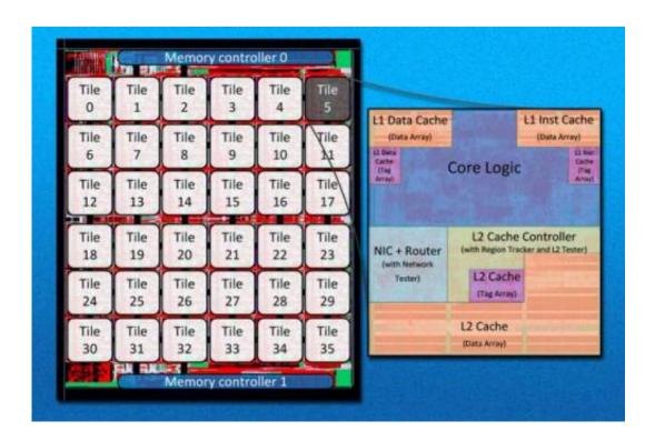
The MIT researchers' new 36-core chip is "tiled," meaning that it simply repeats the same circuit layout 36 times. Tiling makes multicore chips much easier to design.
