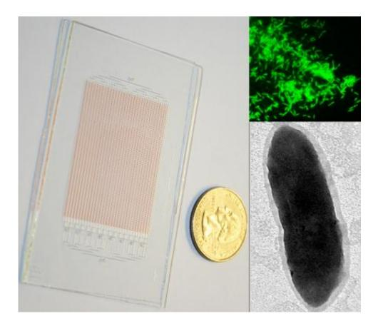
Photograph of a glass SlipChip for growing microbes, shown next to a US quarter (left). Fluorescent in situ hybridization image of the target organism (right, top). Transmission electron microscopy image of a single cell of the target organism (right, bottom). Credit: Liang Ma (Ismagilov group) and Roland Hatzenpichler/Caltech
