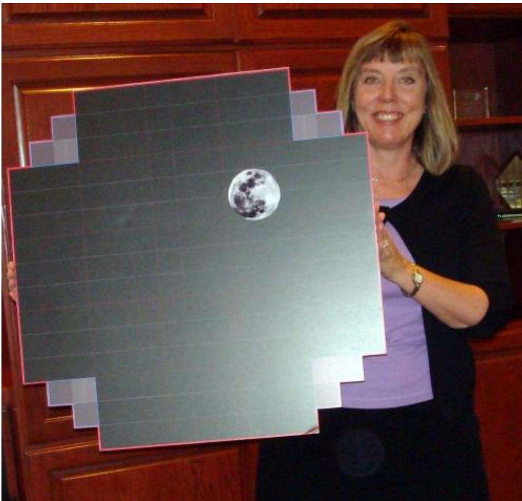
Suzanne Jacoby with the LSST focal plane array scale model. The array's diameter is 64 cm. This mosaic will provide over 3 Gigapixels per image. The image of the moon (30 arcminutes) is placed there for scale of the Field of View. Credit: LSSTC
