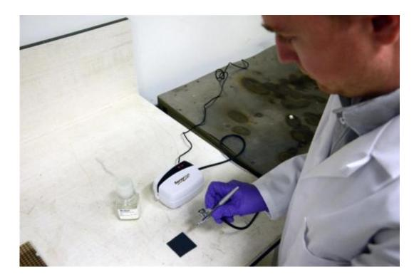
Dr Jon Major demonstrates the new simple method of applying magnesium chloride. Credit: University of Liverpool
