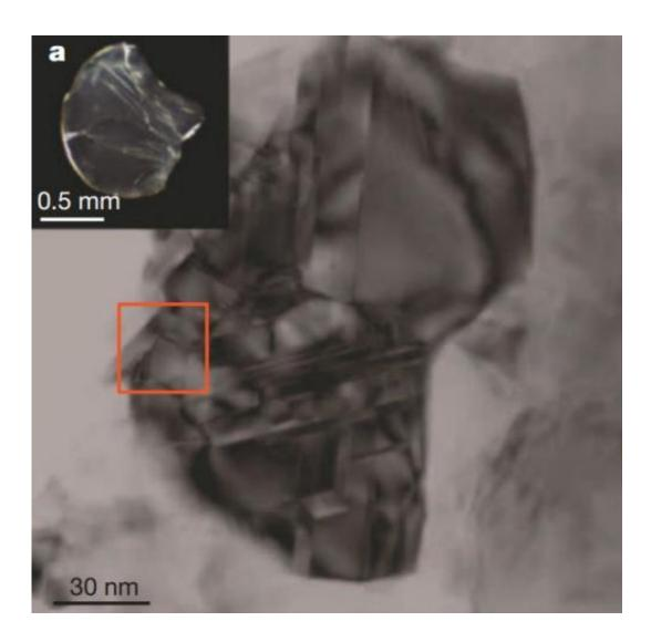
A nt-diamond bulk sample synthesized at 20 GPa and 2,000 C. TEM image of nanotwinned microstructure. Inset: photograph of the transparent sample (1 mm in diameter). Credit: *Nature*, http://dx.doi.org/10.1038/nature13381
