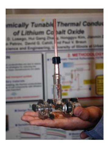
The in-situ TDTR liquid cell is composed of  $LiCoO_2$  thin film cathode, a Li anode, and liquid electrolyte. Credit: University of Illinois
