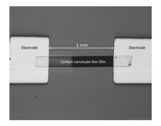
This photograph depicts the terahertz detector developed by researchers at Sandia National Laboratories, Rice University and the Tokyo Institute of Technology. The terahertz radiation is captured by a carbon nanotube thin film contacted by two gold electrodes. Credit: Rice University
