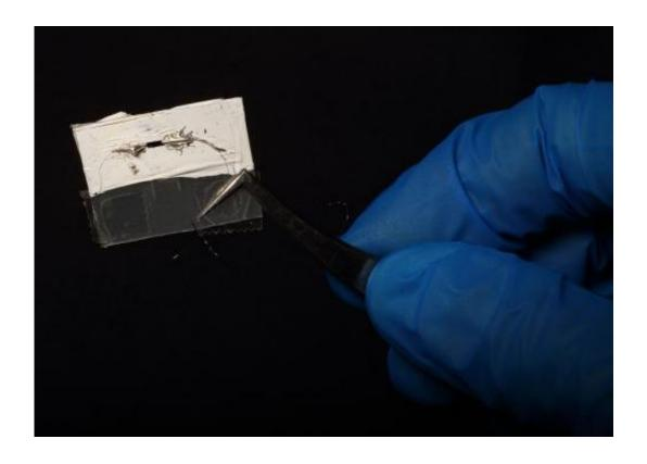
Researchers at Sandia National Laboratories, Rice University and the Tokyo Institute of Technology developed a terahertz detector using several nanoscopic-sized tubes, creating a macroscopic thin film that contains a mix of metallic and semiconducting carbon nanotubes. Credit: Dino Vournas, Sandia National Laboratories
