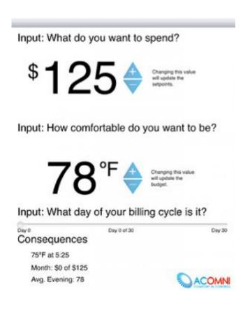
An interface for the cost-limiting temperature-control device advises users of electricity costs for thermostat settings.
