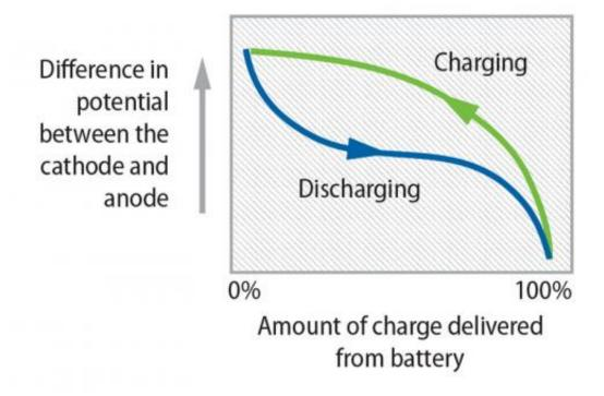
In a rechargeable battery, such as a lithium-ion battery, at maximum potential difference, the battery is fully charged and ready to provide power to a load. And when the potential difference is zero, the battery is fully spent and ready to be recharged. Credit: Joelynn Schroeder, NREL
