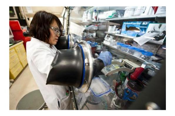
NREL Scientist Chunmei Ban assembles a lithium-ion battery in the materials lab at the Solar Energy Research Facility at NREL. Credit: Dennis Schroeder, NREL
