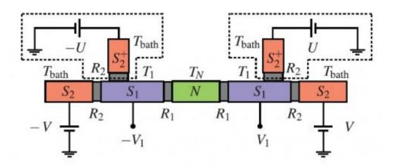
The superconducting cascade electron refrigerator, with a S2IS1INIS1IS2 configuration, can cool a metal from 0.5 K to 100 mK in a cascading two-step process. Credit: M. Camarasa-Gómez, et al. ©2014 AIP Publishing LLC
