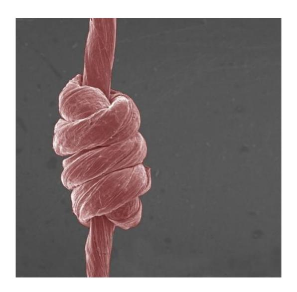
Strong, stretchable fibers made of graphene oxide can be knotted like yarn. Credit: Terrones group/Penn State
