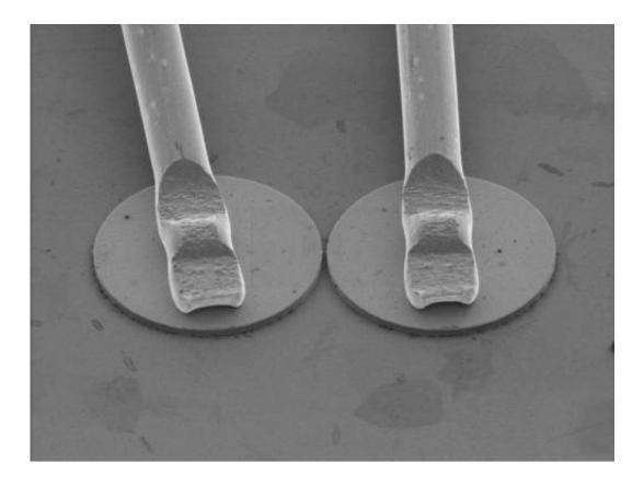
An electron microscope image shows two lasers placed just two microns apart from each other. Credit: Vienna University of Technology
