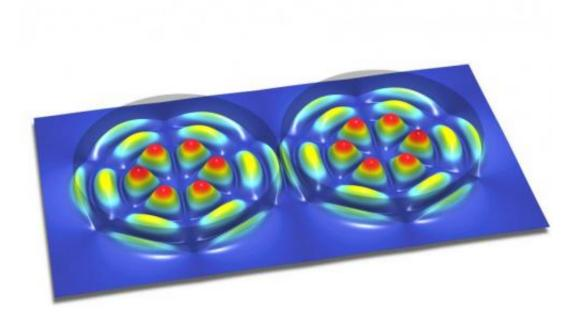
Manipulating minute areas of gain and loss within individual lasers (shown as peaks and valleys in the image), researchers were able to create paradoxical interactions between two nearby lasers. Credit: Vienna University of Technology
