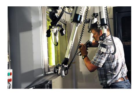
Irradiated nickel-based alloy specimens loaded into new test rigs at INL's Materials and Fuels Complex marked the next stage in a series of experiments with industry research partners through the ATR National Scientific User Facility at INL.
