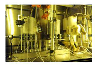
Irradiation-Assisted Stress Corrosion Cracking test rigs allow researchers to gather data on the growth of cracks in highly radioactive compact tension (CT) specimens.
