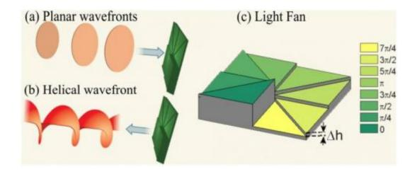
(a) The normal incident laser pulse has a planar (non-twisted) wave front.(b) After reflecting off of a spiral foil, the light has a helical (twisted) wave front.(c) The foil used in the simulation has eight parts to mimic a spiral phase plate.Credit: Shi, et al. ©2014 American Physical Society
