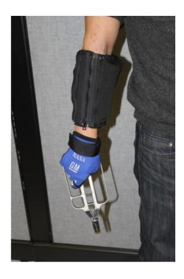
This is a demonstration of RoboGlove providing assistance with a grasping task. Credit: NASA
