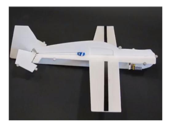
A team of CSAIL researchers designed a single-motor glider (pictured here) that can perch on power lines like a bird.
