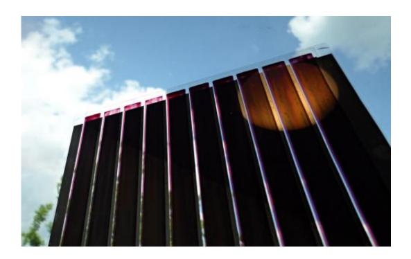
Organic photovoltaics printed on ultra-thin glass. Credit: Fraunhofer IAP
